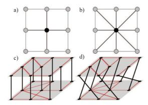
Fig. 1: (Color online) Considered network topologies. Panel (a) shows the scenario of a monolayer network with nearest-neighbor interactions (k=4), whereas panel (b) shows the case where the next-nearest neighbor interactions are also included (k=8). Panel (c) shows results for the multiplex two-layer network, whereas panel (d) shows results when there is random connectivity between the two layers.
